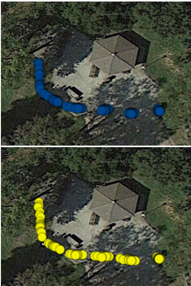
Figure 8: Fixed RTK positions – ProMark 220 in blue (top) and competitive product in yellow (bottom), when a competitive brand base is used.
