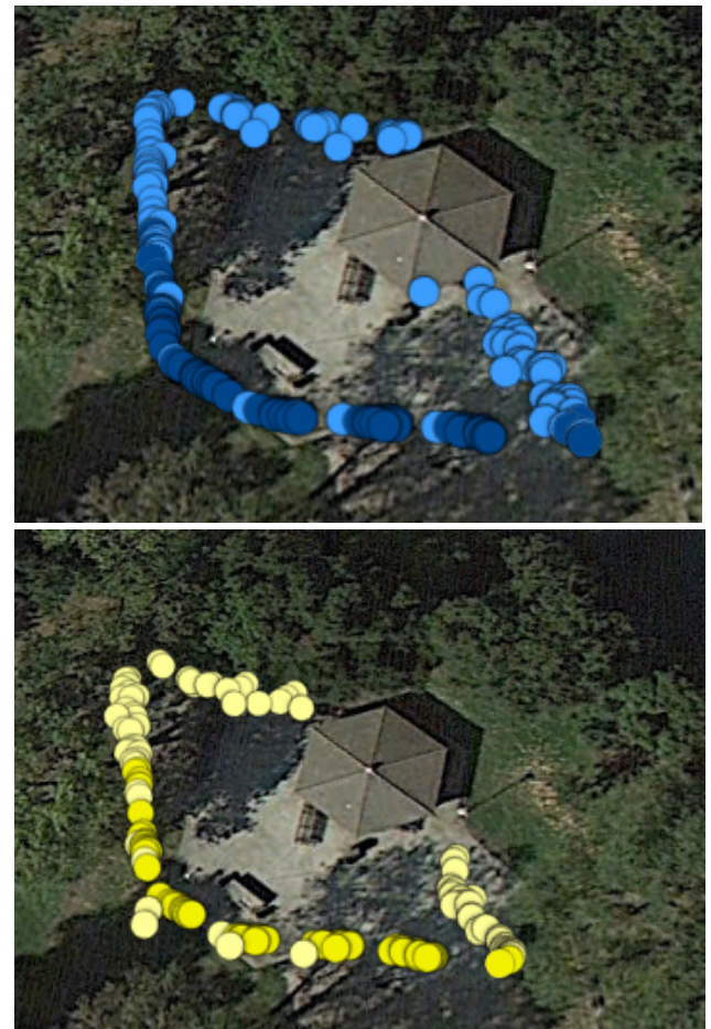
Figure 9: Fixed RTK and float positions – ProMark 220 in blue (top) and competitive product in yellow (bottom), when a competitive brand base is used.
